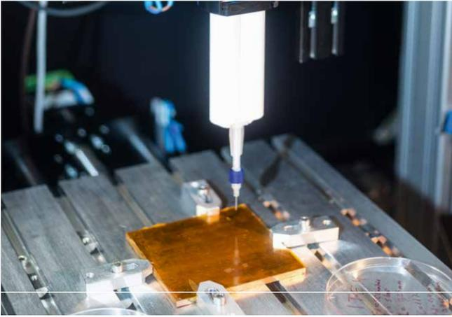
*The custom-developed 3D printer enables processing of medical-grade silicone rubber and conductor materials to produce individualized neural implants.*
