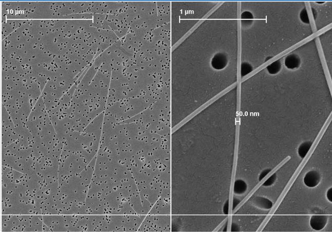
*To date, there is hardly any toxicological data available for fibrous innovative nanomaterials such as the silver nanowires shown here (SEM image). The aim of the project MetalSafety is to develop an in-vitro model for the toxicological evaluation of different metal-based compounds that differ in bioavailability.*
