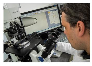
Picture 1: Under the microscope, Bernhard Polzer isolates single cancer cells he previously obtained from patient material. The monitor shows the glass capillary with the cell he previously identified as a cancer cell and then suctioned off the slide.
