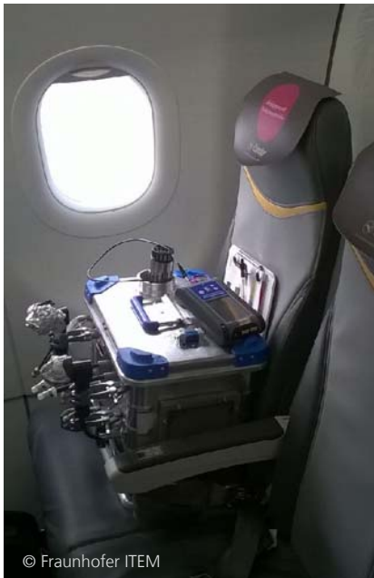
© Fraunhofer ITEM Sampling box for in-flight measurements.
